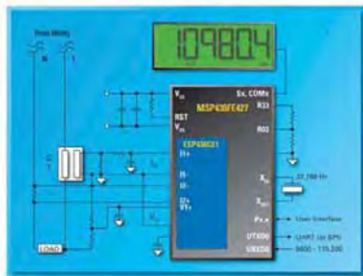
Figure 3. AMR-ready single-phase e-meter with anti-tampering functionality
