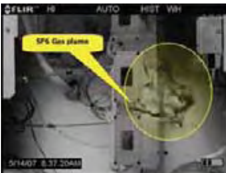
Figure 5. SF 6 leaking from a cracked bellows on a governor switch.
