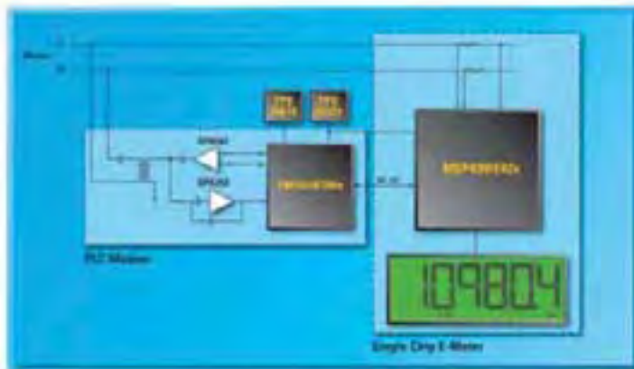
Figure 1. PLC-based AMR dual-chip e-meter solution by TI
