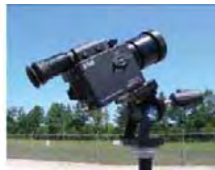
Figure 1. GasFindIR LW viewing rupture disks on 500 KV live switchgear. Inset at right shows the GasFindIR mounted on tripod to exploit high sensitivity mode.
