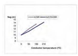
Fig. 2. Sag in function of the conductor temperature for a span length of 400m
