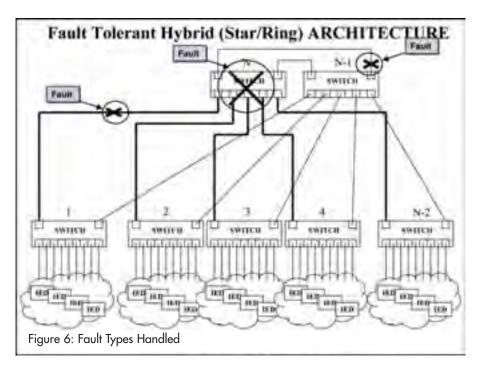
switches connected to the backbone switch N.
