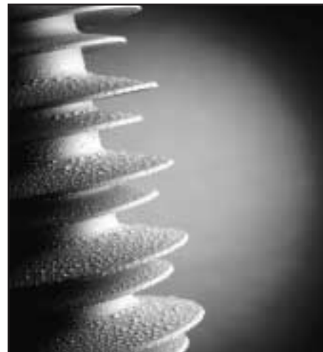
Water droplets on a polymer arrester housing. Current is not conducted as easily as on a porcelain housing, where the water spreads out to form a uniform layer.
