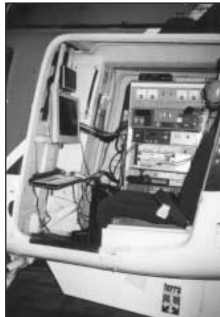
Configuration of LIDAR mounted to Bell helicopter
