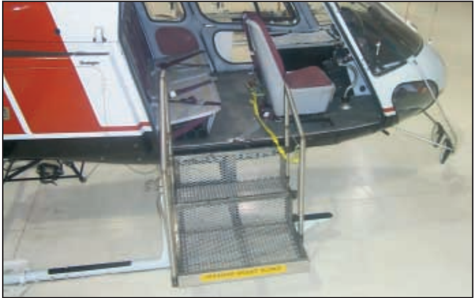
The concept was named 'AirStair' and was attached to a Eurocopter AS 350B2, AStar helicopter.
