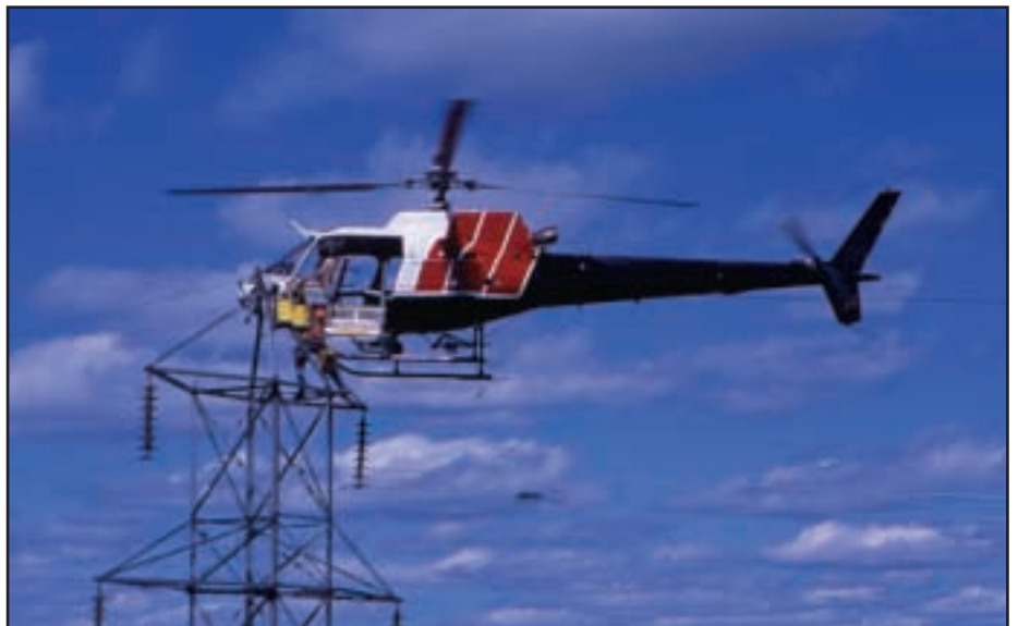
The concept was named 'AirStair' and was attached to a Eurocopter AS 350B2, AStar helicopter.
