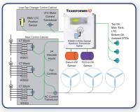
The **TransformeriQ** PLC-based platform replaces traditional IEDs and single functional sensors to provide centralized monitoring. The system controls and logs a variety of performance parameters including LTC position history, LTC motor operation, multi-stage cooling, gas-in-oil, and advanced RTD and fiber optic temperature measuring.
