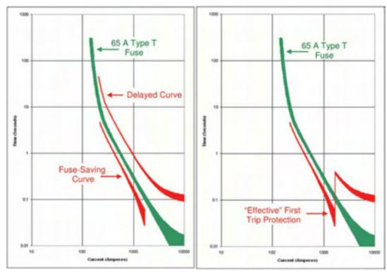
Figure 3. Partial range fuse-saving curve is implemented from the delayed curve minimum trip through the maximum coordinating current.
