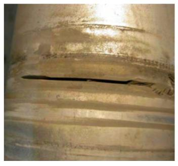
Figure 2 Damage caused by arcing
