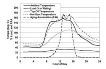
Figure 3 – Loading, thermal behavior, and resulting aging for peak day, Savannah high school load.
