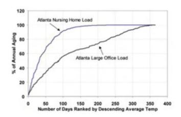
Figure 5 – Comparison of transformer aging histograms
