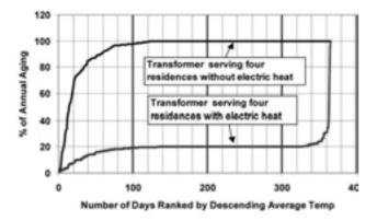
Figure 7 –Aging histograms transformers serving typical four-residence loads, with and without electric space heating
