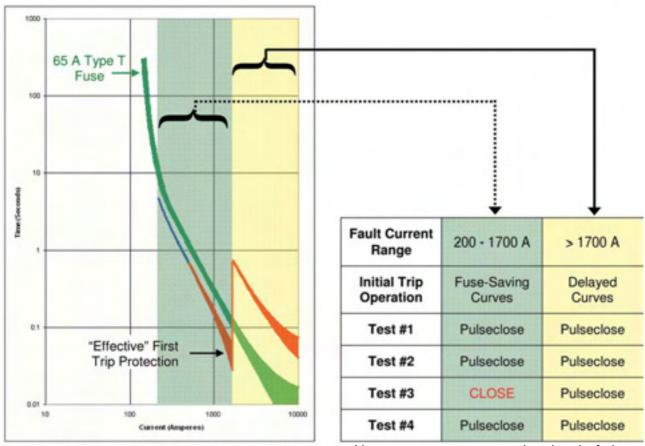
Figure 7. The left shaded area (green) represents the range of effective fuse-saving.
