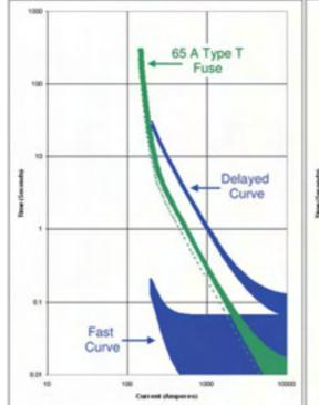
Figure 1. Conventional Fuse-Saving using a common fast TCC curve.
