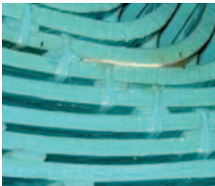
Figure 4: PD occurring between high voltage coils in two different phases, where the spacing is insufficient to prevent the PD. Note that the spacing between adjacent coils is irregular, as a result of poor manufacturing processes.
