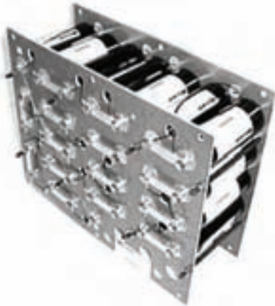
Fig. 6. Internal design of high-voltage (ten voltages) supercapacitor, assembled from number of low-voltage elements
