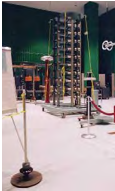
Figure 2. View of the 1000 kV surge generator.
