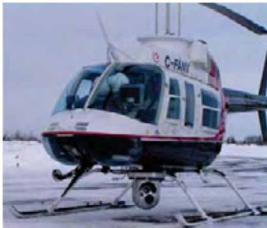
Photos show the Gimbal mounted under the Aircraft. Notice the two monitors so the Pilot and Thermographer can work together. (At right) Work station for the Thermographer. A screen monitor and a field tablet as a second monitor and data collector.
