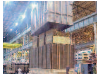
Tank lowered over core and coils
