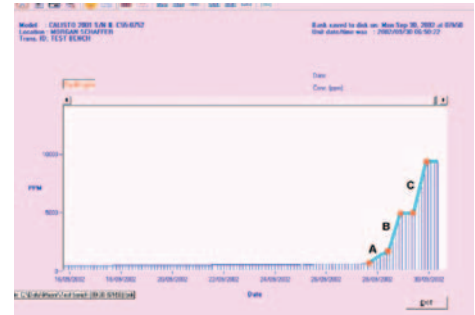
Figure 6: Sudden increase in hydrogen generating rate
