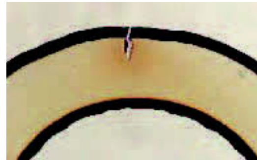
Section of cable with heat damaged insulation
