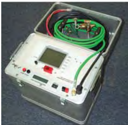
New Saidi Saver Loop Restoration Simultaneously shows distances to each transformer and fault
