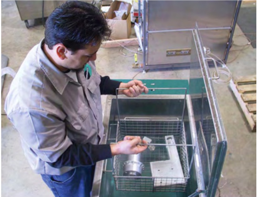
The tanks utilize specialized environmentally friendly but effective cleaning solutions, heat, water, and ultrasonic sound waves for cleaning.
