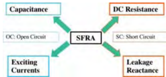
Figure 3 SFRA as part of an Integrated Test Suite
